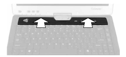
**6** Press down on the bezel in several places to make sure it is correctly mounted. The bezel is correctly mounted when you can run your finger along the bezel and find no loose spots. The bezel should be flat all the way across.
